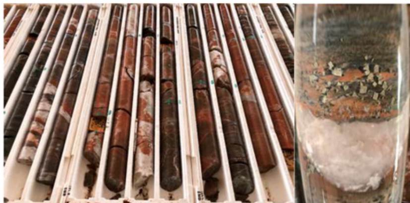
Figure 5: Image showing core from Templar DDH21-3 (results outstanding) which shows hematite altered porphyry with pyrite crystals and sericite alteration overlain with albite alteration. Identical to Karari. Source: NXM
